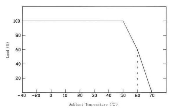
isometry and their life, please refer to the Derating Curve and derate according to the temperature. ■
