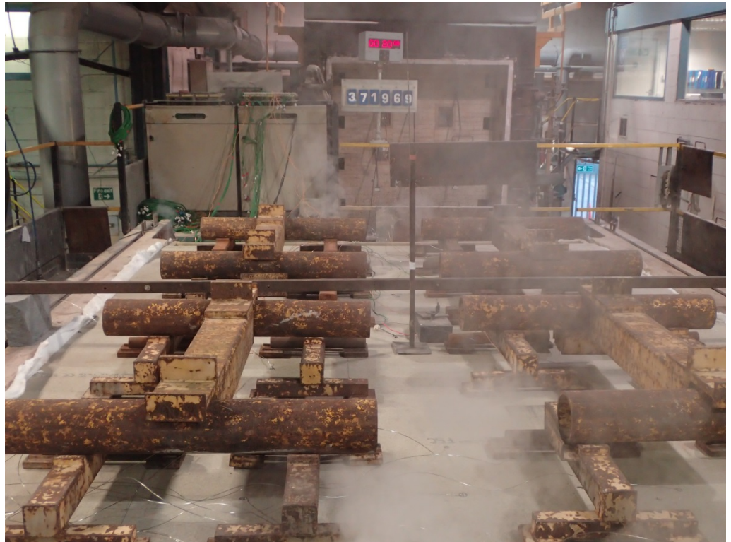
The unexposed face of the assembly after 20 minutes of testing
