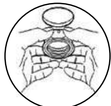
Insert housing. Make sure that the housing is properly seated and level.
