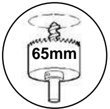
Tools Required- 65mm holesaw. Ceiling will require skim-plastering.
