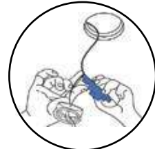
Connect the earth cable on housing to mains connector.
