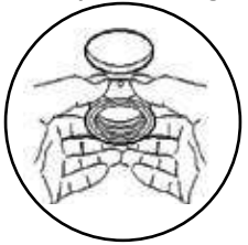
Use Test Housing to check correct fit.
