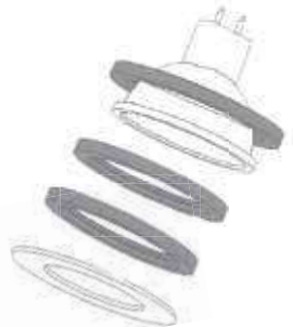
Place lamp in the recess of two magnets.
