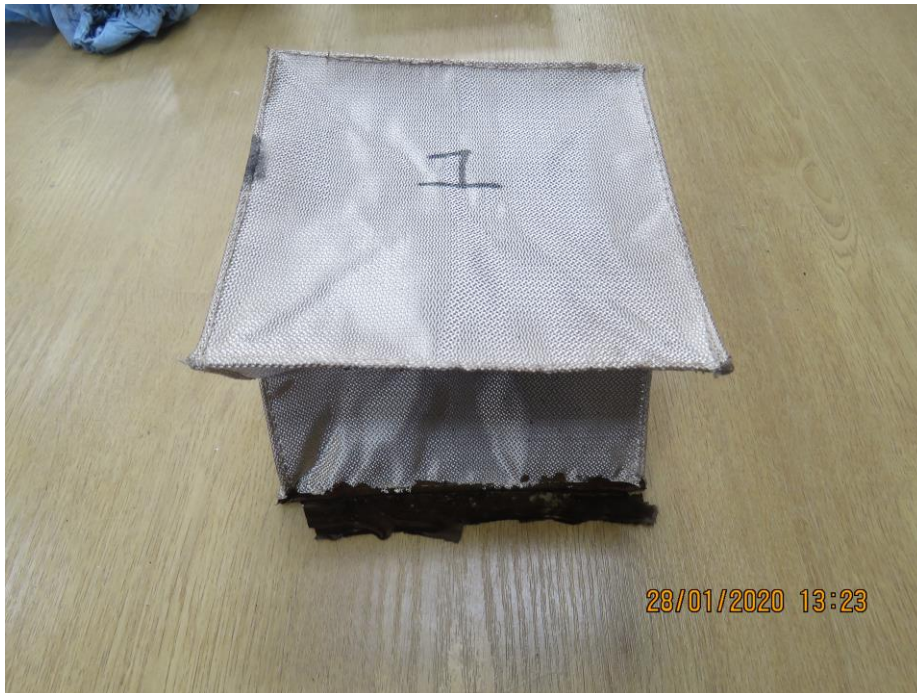
Frame 3: Fire hood 1 post test
