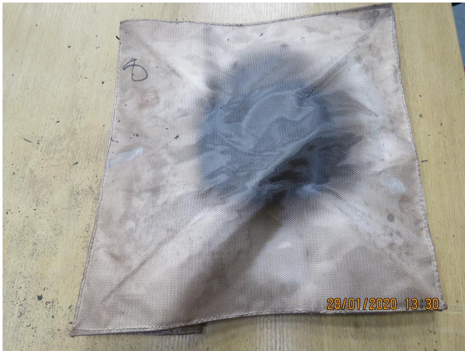
Frame 24: Fire hood 8 post test
