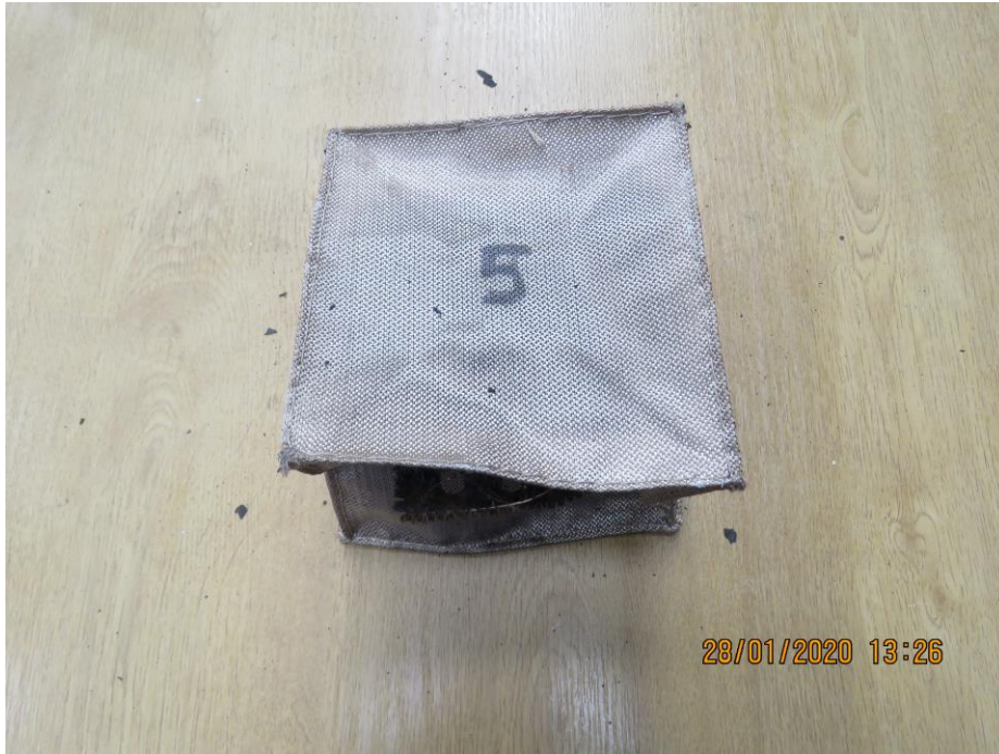
Frame 15: Fire hood 5 post test
