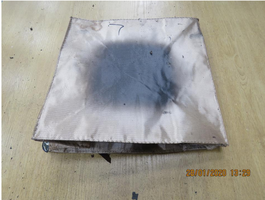
Frame 21: Fire hood 7 post test
