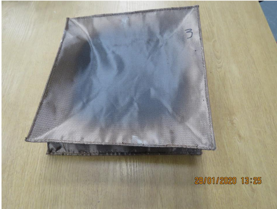
Frame 9: Fire hood 3 post test
