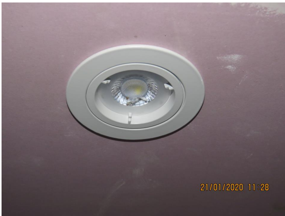
Frame 10: Downlight 4 exposed face pre-test
