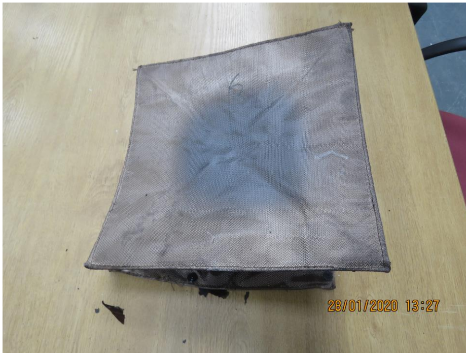
Frame 18: Fire hood 6 post test
