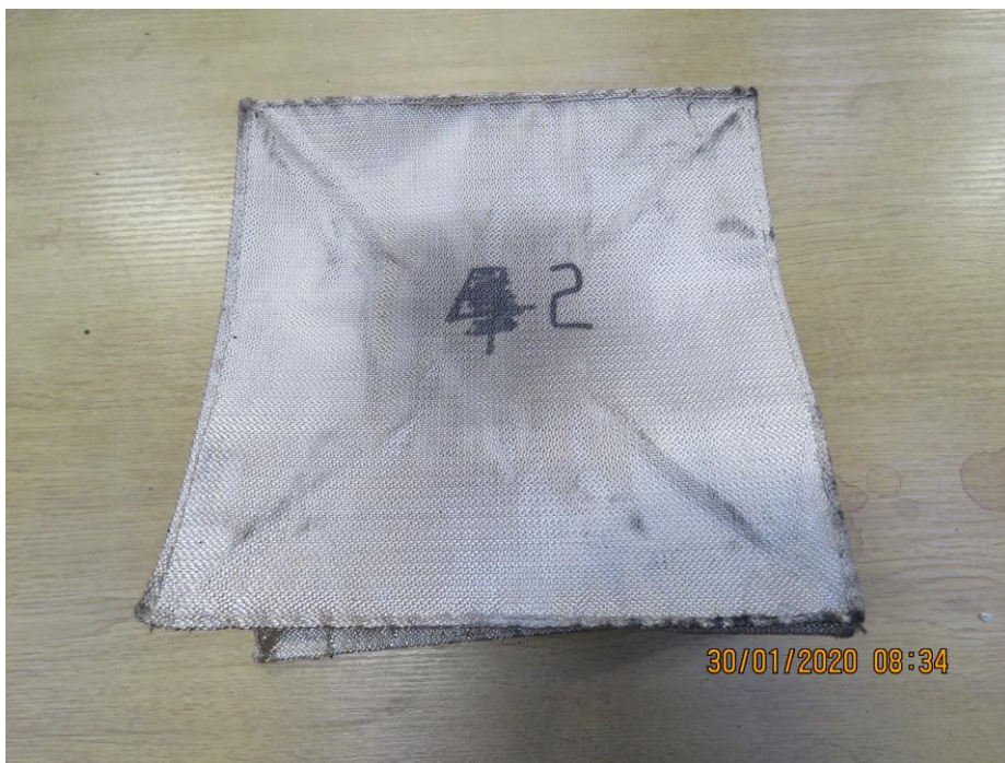
Frame 6: Fire hood 2 post test
